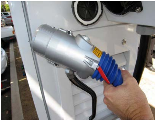
Prototype SAE “Combo” DC Fast Charging Plug
