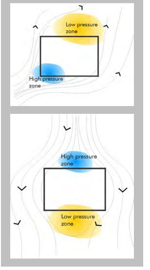
pressure on the leeward side drops, creating pressure stratification across the building. To equalize pressure, outdoor air will enter through available openings on the windward side and eventually be exhausted through the leeward side.
