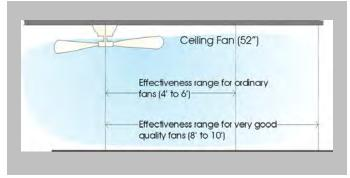
evaporation of moisture from their skin. As long as there is some air movement, people can generally tolerate higher temperatures. Generally, for speeds above 30 fpm, most people will perceive a 15 fpm increase in air to be equal to 1°F decrease in temperature (this is commonly called "chill factor").
