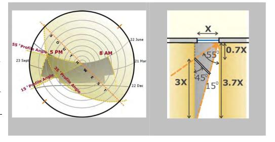
In summary, a combination of overhangs and vertical fins will provide adequate shading for southwest windows in Hawaii.
