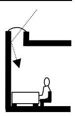
baffles and reflective, matte light well and interior wall surfaces help diffuse the daylight.
