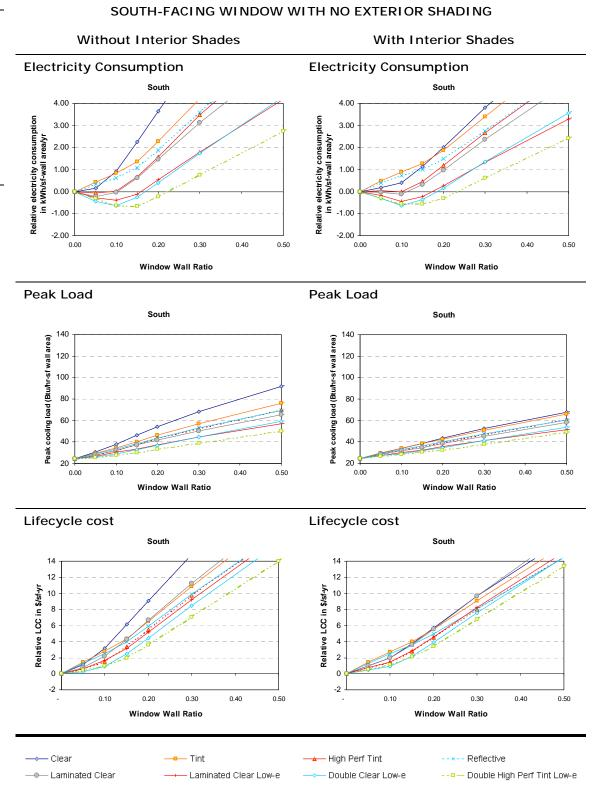
Figure 5-51. South window. Overhang PF = 0.25.Impact of WWR on electricity consumption, peak load demand, and lifecycle cost.
