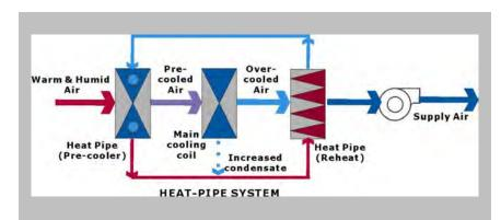
exchanger it vaporizes the refrigerant and is precooled. This allows the coil to more effectively cool the air to a point below the dew-point temperature and to extract more moisture. The air then passes through the second heat exchanger and is reheated, which liquefies the refrigerant, causing it to flow back to the first heat exchanger. The heat pipe system is hermetically sealed, uses a wicking action, and requires no pump.
