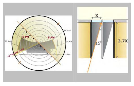
Combining the overhang (35-degree cut-off angle) with vertical fins (15-degree cut-off angle) would provide complete shading between 8 AM and 5 PM, as shown in Figure 5-20. This combination of vertical fins and overhangs is sometimes called an "egg crate" design.
