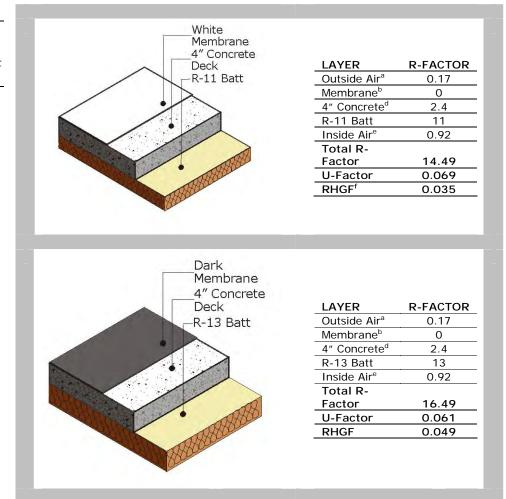
Figure 6-8: Lowslope metal deck roof assembly
