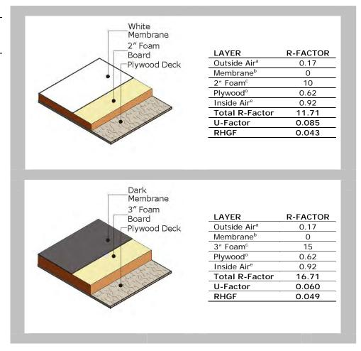
Figure 6-12: (cont'd.) Low-slope plywood deck roof assembly
