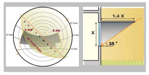
Figure 5-19 shows when the southwest window will be shaded by vertical fins with a 15-degree cut-off angle (equal to a projection factor of 3.7).
