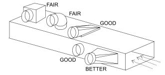
The fewer turns the better. For example, a side branch takeoff provides less flow resistance than a top branch takeoff because the top takeoff requires the air to turn twice.
