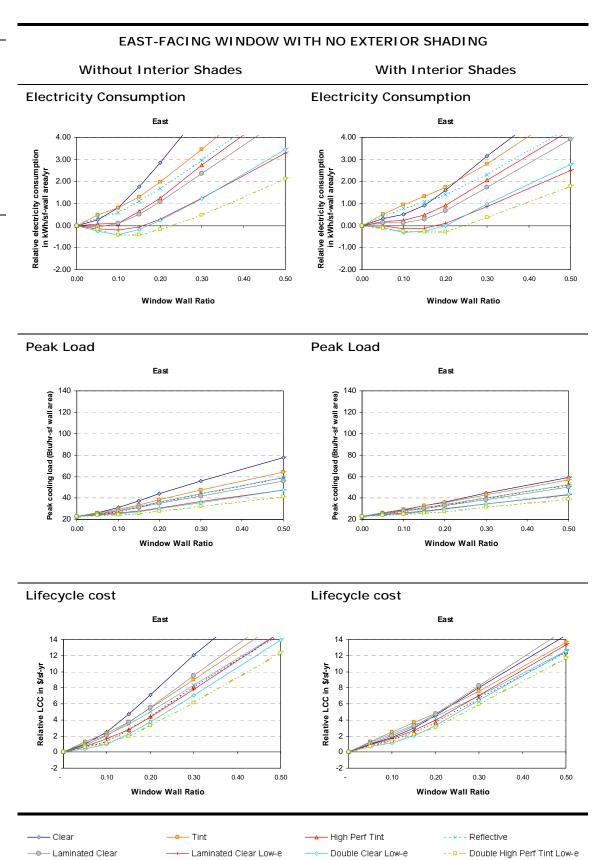
Figure 5-43. East window. Overhang PF = 0.25. Impact of WWR on electricity consumption, peak load demand, and lifecycle cost.
