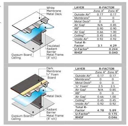
Figure 6-10: (cont'd.) Low-slope metal deck roof assembly
