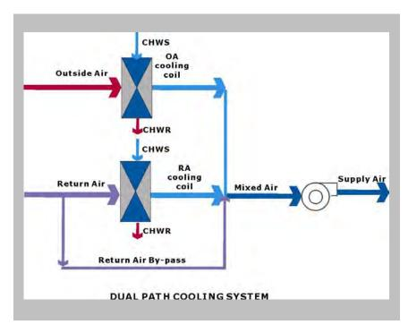
In chilled water dual-path systems, the outdoor air (OA) coil can use cold chilled water at 40°F to 42°F for latent cooling, while the return air (RA) coil can use warmer chilled water at 50°F to 60°F for sensible cooling, thus improving chiller efficiency. Dual-path systems decouple the sensible cooling and latent cooling of the supply air, thereby improving control of temperature and humidity.
