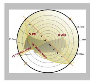
Shading devices can be designed in several ways, as long as the relationship between the window height and the depth of the shading device (the cut-off angle) does not change.
