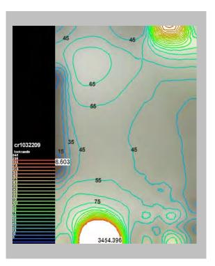
Figure 5-10. Radiance image showing threedimensional view of corner window for a specific time and day. Source: Eley Associates.
