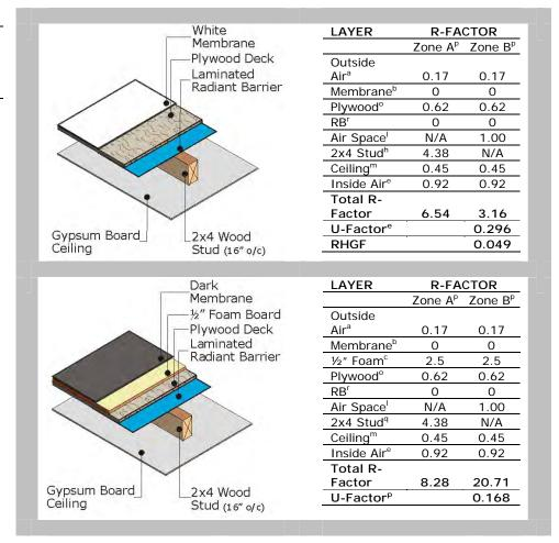
Figure 6-14: (cont'd.) Low-slope plywood deck roof assembly
