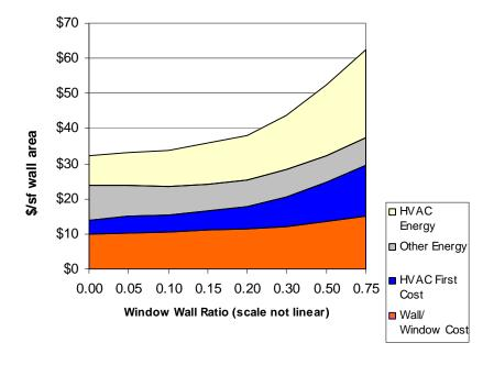
Figure 5-4 shows the lifecycle cost for one case: single-pane, high-performance tint in a south-facing window. The "other energy" decreases gradually until the WWR reaches about 0.20, while the other components of lifecycle cost increase slightly. The net result is a gradual increase in the lifecycle cost up to about 0.20 WWR.
