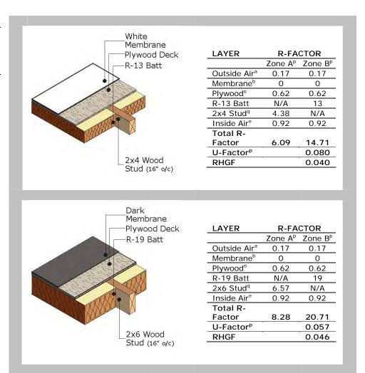
Figure 6-13: (cont'd.) Low-slope plywood deck roof assembly
