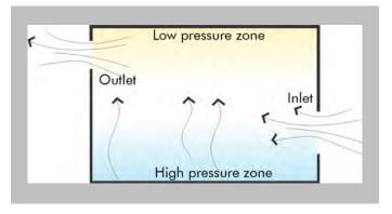
ventilation to occur. Higher indoor temperatures cause a pressure difference so that the upper openings act as the outlet and cool air intake is induced at the lower opening.
