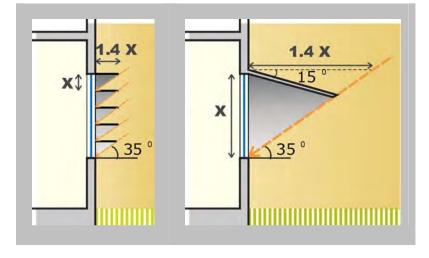
Figure 5-23. Plan view showing alternative design for vertical fins. Note that the cutoff angle remains unchanged.
