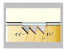
Figure 5-20 above shows that there is a certain amount of overlap between the period shaded by the horizontal overhang and that shaded by the vertical fins. Thus, there is some redundancy in this solution. As shown in Figure 5-24, additional shading is required only when the sun is between an angle of 15
