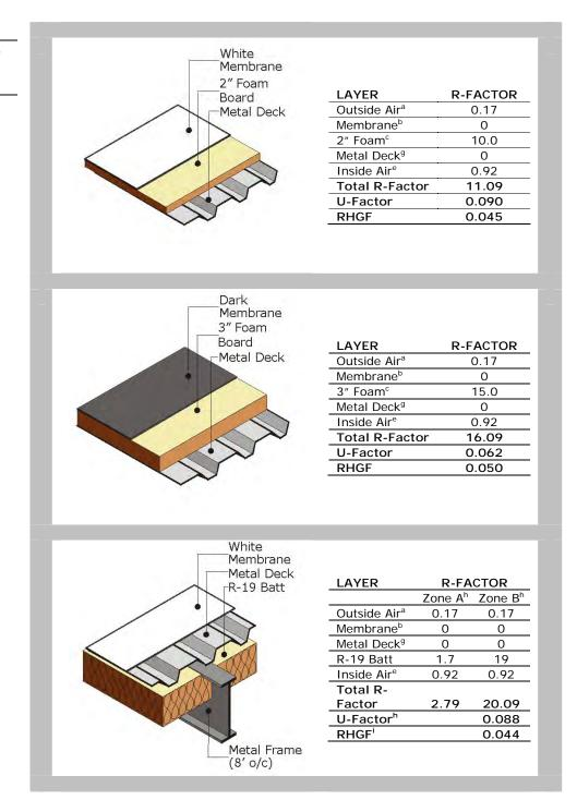
Figure 6-9: (cont'd.) Low-slope metal deck roof assembly
