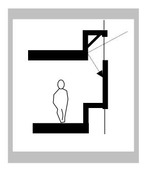
**Shading devices:** Use exterior shading devices, diffusing glazing, operable blinds, lightshelves or louvers to reduce or eliminate direct sun penetration. The following guideline, High Sidelighting — Clerestory with Lightshelf or Louvers, discusses the lightshelf and louver strategies. The Energy-Efficient Windows Guidelines provide information about the appropriate depth of exterior shading devices.
