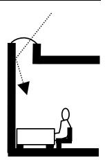
baffles and reflective, matte light well and interior wall surfaces help diffuse the daylight.
