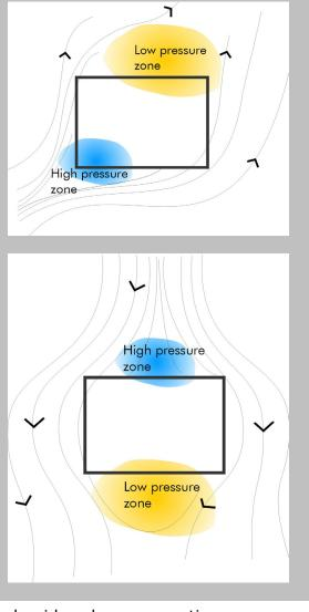
pressure on the leeward side drops, creating pressure stratification across the building. To equalize pressure, outdoor air will enter through available openings on the windward side and eventually be exhausted through the leeward side.
