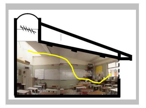
Electric lights are circuited parallel to the view windows and toplit walls, and were originally designed with automatic daylight dimming controls. However, over the years many of these controls
