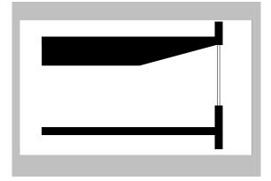
**Integration with HVAC:** High sidelighting can affect a building's overall HVAC loads because it is susceptible to solar gain in the cooling season and heat loss in the heating season. Reduce HVAC loads by correctly orienting the glazing, designing appropriately sized windows, selecting appropriate glazing materials, providing shading, and controlling the electric lighting system. In addition to saving energy, these measures may help to reduce the size and first cost of the HVAC equipment.
