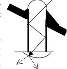
Because they depend on multiple reflections to deliver daylight to the space, tubular skylights perform significantly better in clear sky conditions than in overcast climates. The longer the duct, the less daylight is delivered;
