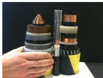
The 200 MW HVDC cable bundle is no more than 10 inches in diameter.
