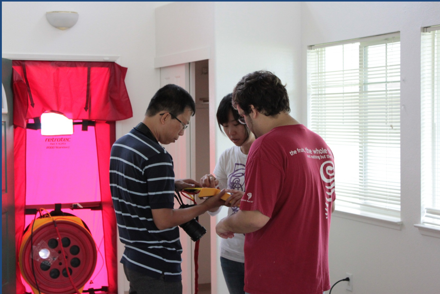
Blower door and duct testing on empty houses
