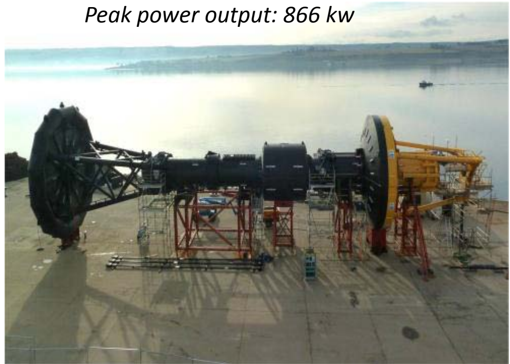
PB150 assembled on wharf
