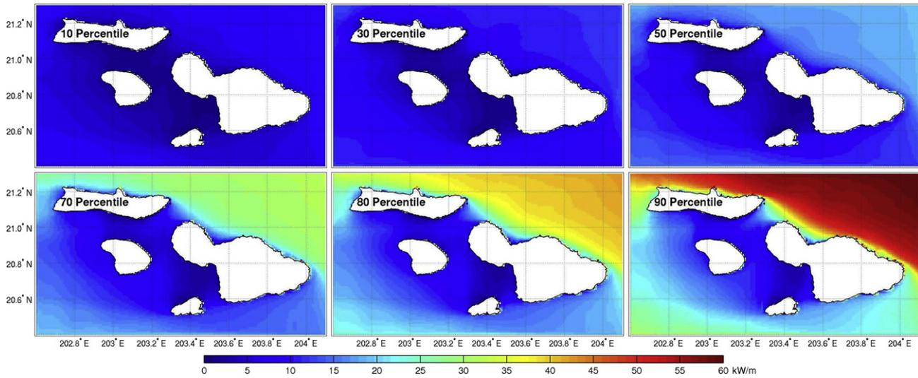
Fig. 18. Percentiles of wave power for Maui.
