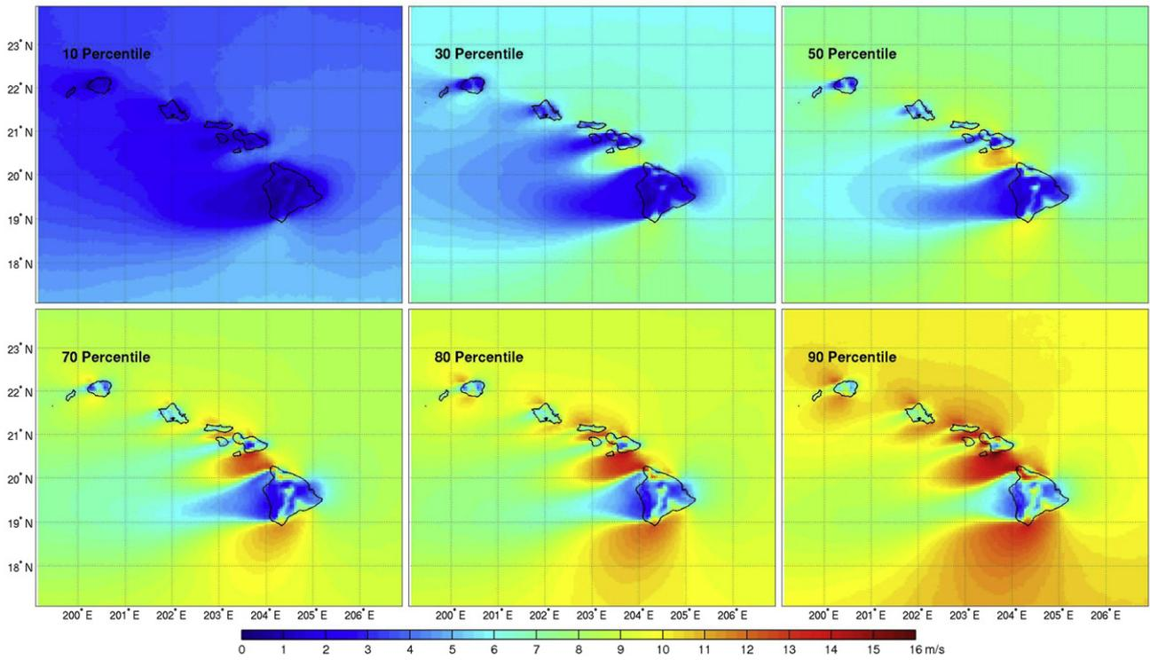
Fig. 4. Percentiles of wind speed from Hawaii WRF.
