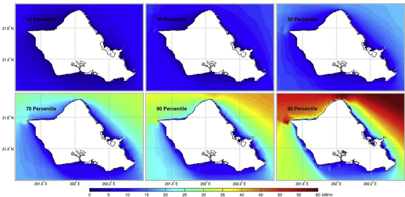
Fig. 17. Percentiles of wave power for Oahu.
