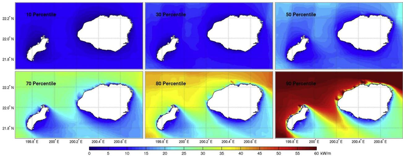
Fig. 16. Percentiles of wave power for Kauai.
