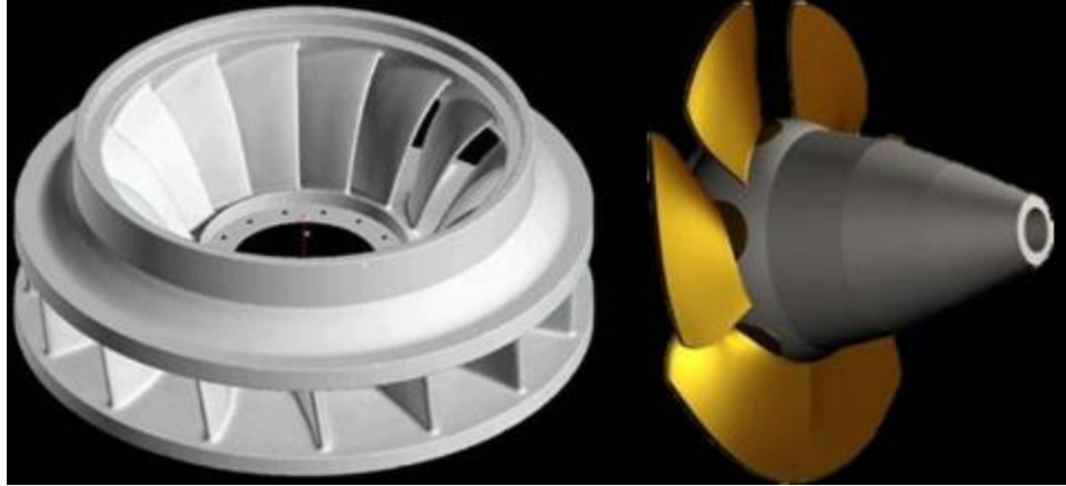
Figure 2-25. Illustration of Francis (left) and Kaplan (right) Turbines (Sources: Topomatika 2013 ; Orengine 2013 )
