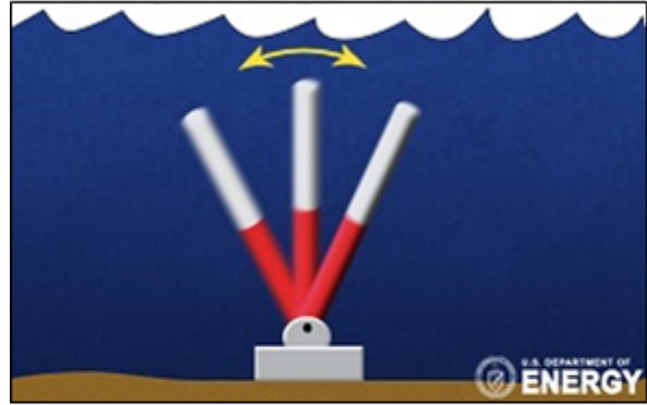
Figure 2-31. Illustration of Oscillating Wave Surge Converter Technology
