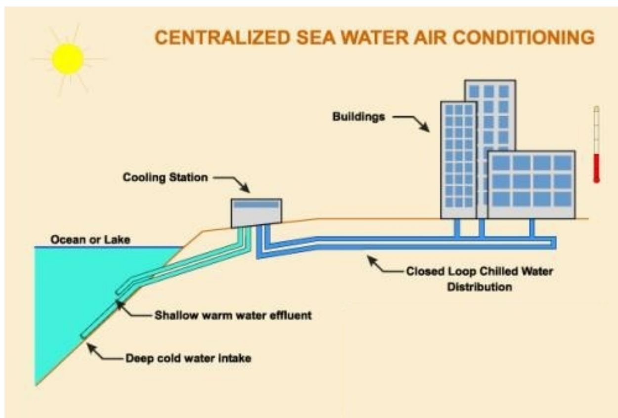
Figure 2-7. Illustration of a Deep Water Cooling Facility ( Source: Makai 2013 )
