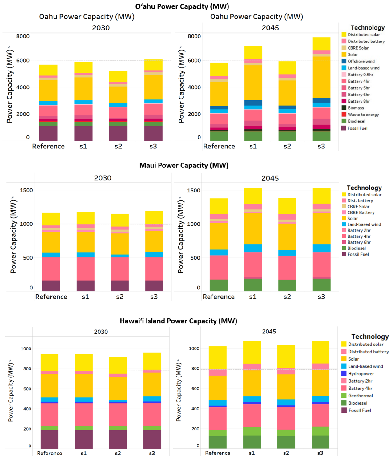
Figure 64. O'ahu, Maui, and Hawai'i Island 2030 and 2045 electric sector generation technology mixes. Distributed battery resources have an average 2.7-hour storage duration.
