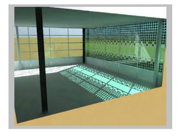
Figure 5-11. Heliodon. Photo: Robert Marcial, Pacific Energy Center. A heliodon can be used to simulate sunlight penetration and shading for a physical scale model of a building. A heliodon is an articulated table that can be adjusted to simulate the position of the sun at any time of the year for any latitude.
