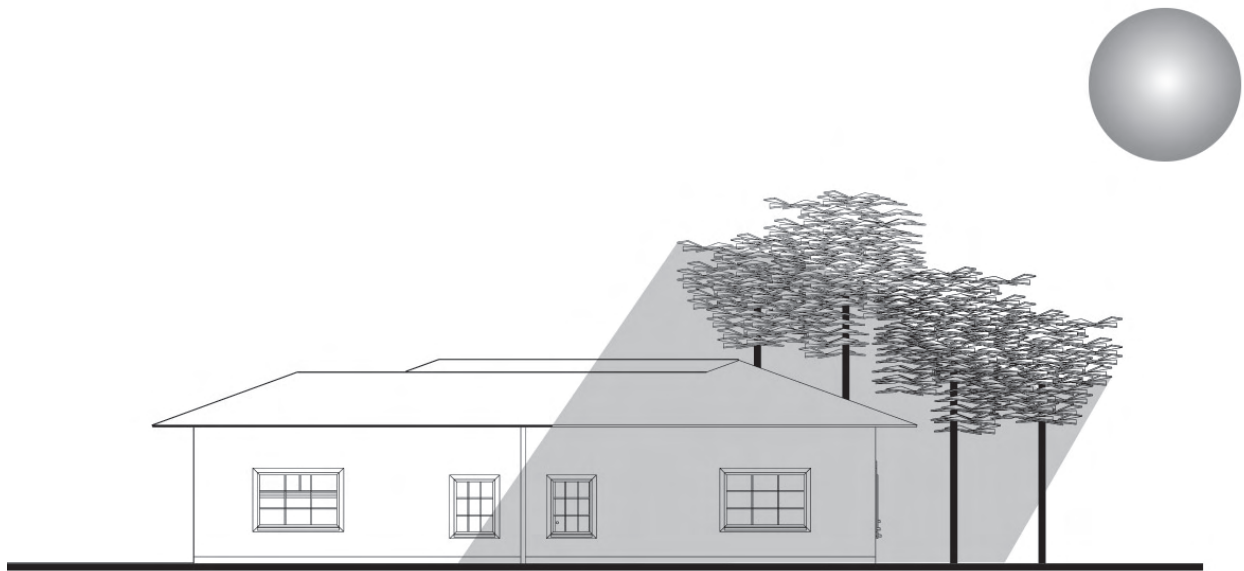
Fig. 8-1: Preventing Heat Gain by Shading the Roof.
