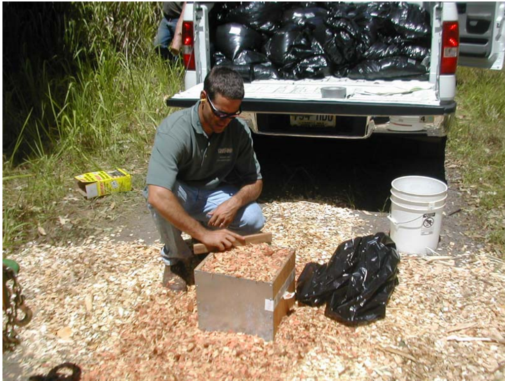
Figure 3. Measurement of bulk density according to ASTM 873 [3].
