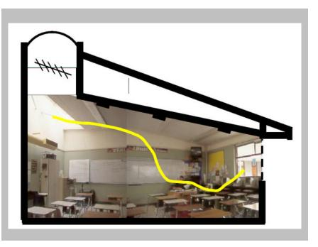
Electric lights are circuited parallel to the view windows and toplit walls, and were originally designed with automatic daylight dimming controls. However, over the years many of these controls
