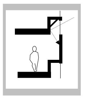
Figure 3-12. Clerestories in multistory buildings can redirect daylight onto the perimeter wall to brighten it.
