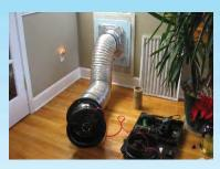
Leakage ≤ 4 cfm/100 ft<sup>2</sup>
