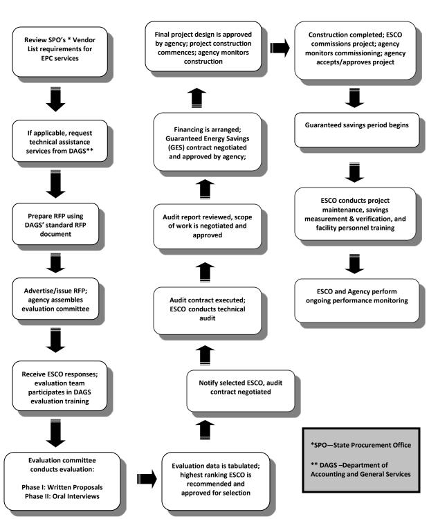
Figure 4-3 Energy Performance Contracting Process Flowchart
